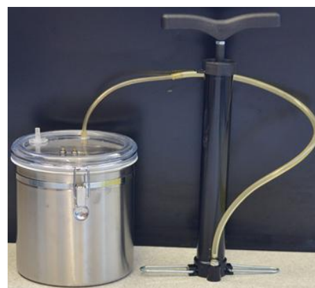
Figure 6: The portable vacuum comprised of a canister (left) and a hand pump (right), constructed to replace the house vacuum.
